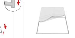
Step 5: Push banner stand frame onto posts of flat base or optional feet. Press evenly on both sides to
